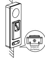
6.Tighten the screws on the bottom of the terminal to fix the terminal on the mounting plate and complete the installation.
