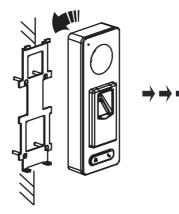
5.Push the terminal in the mounting plate from bottom up.
